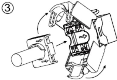
③ Install the termination cap to outlet, which will also allocate the conductors sitting on the slots.
