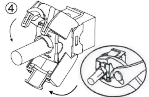
④ Secure the hinged outlet by using a crimp tool until it completely snaps to effect the connection.
