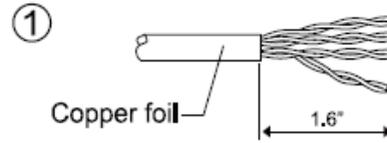
① Strip off 1.6 inch of a cable jacket and fold braid back over it. Cut off aluminum foil for each pair, and use a supplied copper foil shield surrounding a cable.
