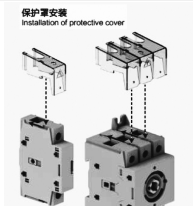
Figure 28 Installation diagram of terminal cover
