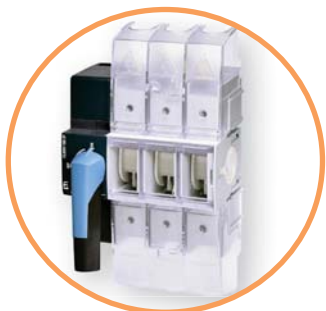
→ Terminal covers provide protection against accidental contact and phase separation of the switch, and Perforated holes allow for contact temperature monitoring without removing the covers
