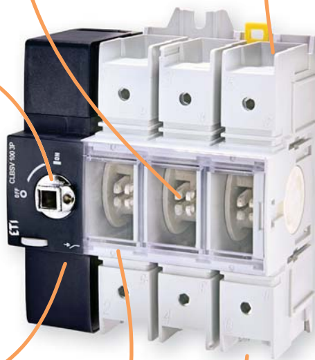
→ Terminal covers provide protection against accidental contact and phase separation of the switch, and Perforated holes allow for contact temperature monitoring without removing the covers
