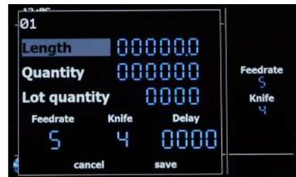
Now enter the desired length of the blank. The entry is made in mm with one decimal place. By turning the navigator, move between the digits of the input and change them by selecting (pressure) and adjusting (rotation). Please enter a 2 for the hundredth place and a 5 for the tens.
