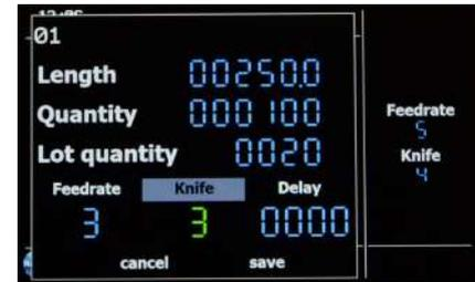
The delay is programmed to the value 50. This causes the feed to be slowly accelerated at the beginning and gently slowed down at the end.
