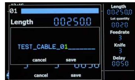
The values are now stored under the program number. The display now shows the following picture. By selecting the program number you can start the cutting process or change the programmed values. Go to the menu item Change.
