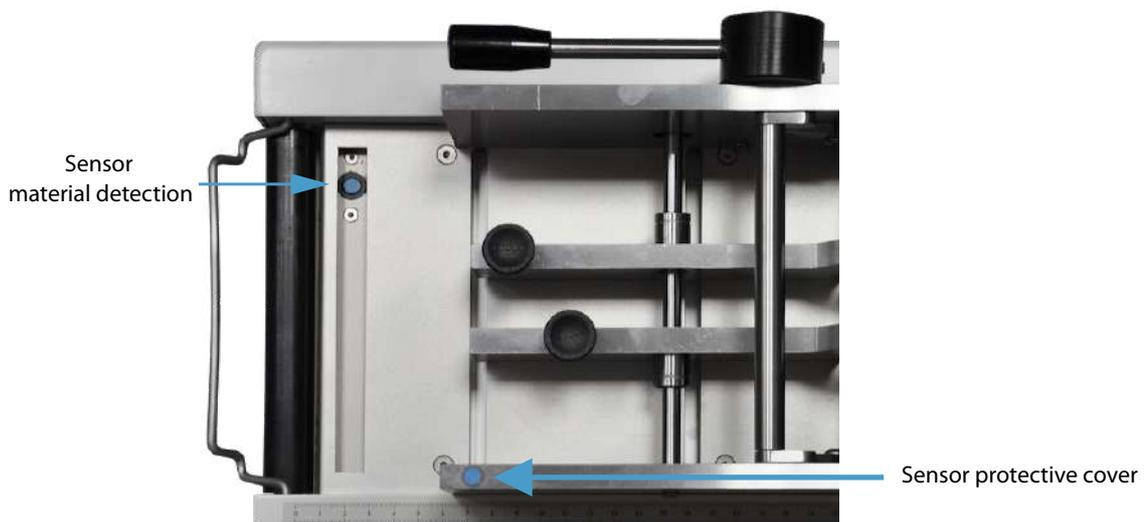
The machine can not be started when the protective cover is open. A corresponding error message will be shown on the display.
